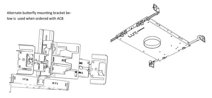
Open Frame [OF], Insulated Ceiling [IC] or, Chicago Plenum [CP] versions will FIRST install ceiling pans [shown above] in plenum prior to fitting ceiling material about fixture aperture.
