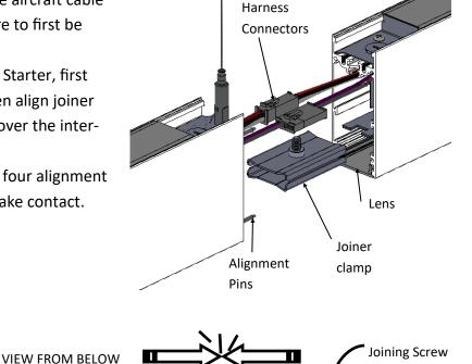
From below, with the lens removed, the joiner bracket screw should be visible and self-centered about the gap between and behind adjacent LED boards. Fasten screws while ensuring that housings are still squarely in contact with each other to complete the joining of each subsequent continuous row fixture. Re-insert lens into its position.
