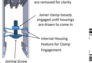
From below, with the lens removed, the joiner bracket screw should be visible and selfcentered about the gap between and behind adjacent LED boards . Fasten screws while ensuring that housings are still squarely in contact with each other to complete the joining of each subsequent continuous row fixture. Re-insert lens into its position.
