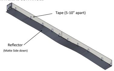
Push Reflector upward and remove tape
