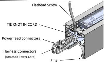
For row mounting fixtures attach male end of harness to female end of harness and slide fixtures together until no gap remains. Fasten flathead screws on each fixture. Fasten reflector tabs down with supplied screws after sliding fixtures together.
