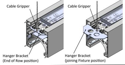
Use provided flathead screws to secure hanger bracket to fixture.
