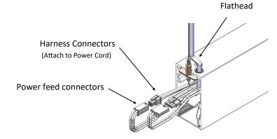
For row mounting fixtures attach male end of harness to female end of harness.
