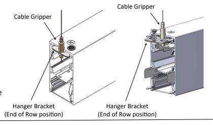
Use provided flathead screws to secure hanger bracket to fixture.
