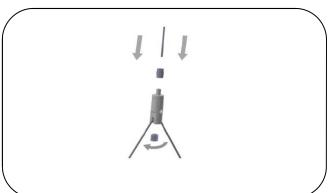
Install "YOKE MOUNT" cable assembly at ends of fixture. Fit assembly into keyway and rotate assembly to be perpendicular with fixture.
