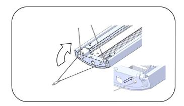
Align fixture to have it straight and level by adjusting the cable.
