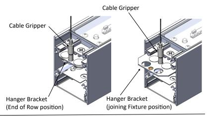
Use provided flathead screws to secure hanger bracket to fixture.
