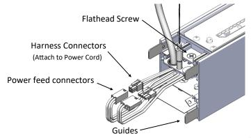
For row mounting fixtures attach male end of harness to female end of harness and slide fixtures together. Small lens section is centered between fixtures to avoid light leak at lens ends.
