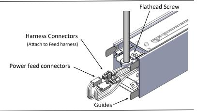
For row mounting fixtures attach male end of harness to female end of harness and slide fixtures together.
