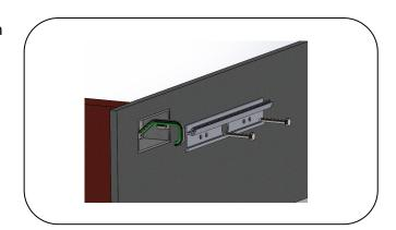
Mount bracket that supports far end of the fixture making sure both brackets are the same height and level. For an 8 foot fixture 3 brackets are included.
