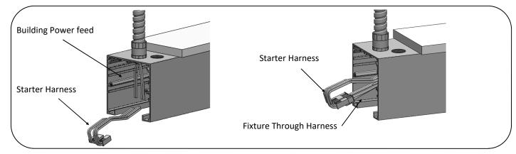
Insert building power feed through housing hole by <u>conduit</u> or <u>Junction box</u> (supplied by others). Splice Building power to "Starter Harness" according to the wiring diagram below.
